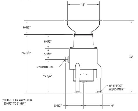
NOTE: Accessory Groups A and B – 18" Cone is Standard. Specify 15" Cone in Place of 18" Cone When Desired.
