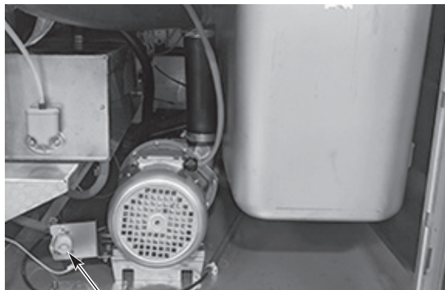
HOT WATER CONNECTION
