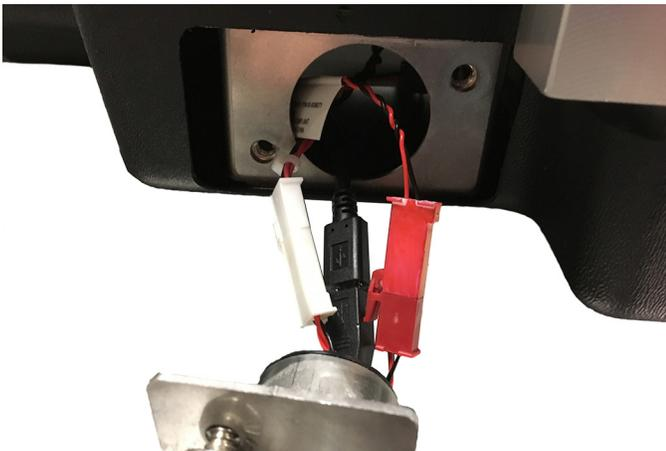
3. Gently insert the display arm tube into the slicer while pushing excess wire length into the machine.
