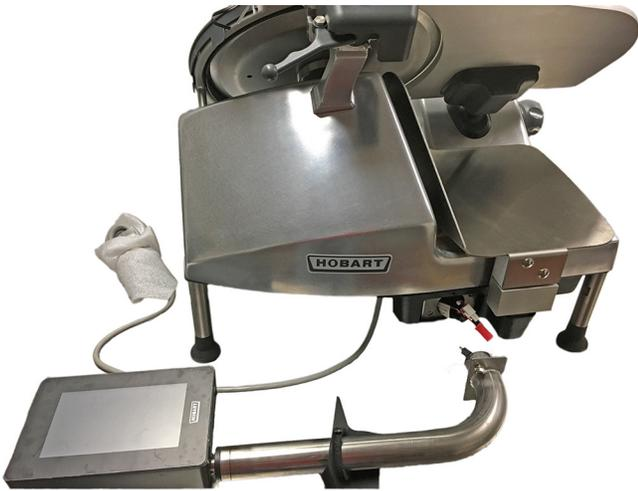
2. Connect the wires from the display arm to the wires coming from the slicer (HS6-1PS shown, HS7-1PS has 4 wires).
