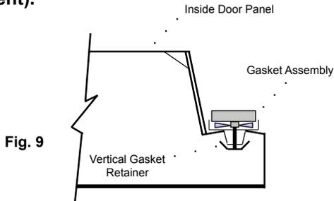
**NOTE:** The gasket may appear too large, but if it is installed as indicated above it will slip into place.
