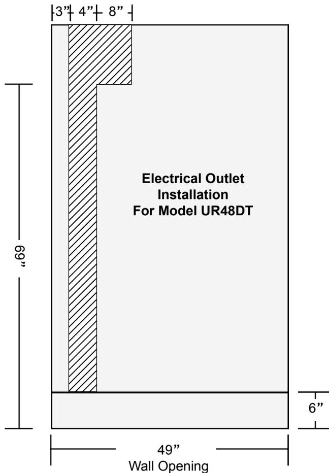
**NOTE:** Wall location of electrical outlet for built-in units and applications that require unit to be counter top depth, locate outlet in shaded area only.
