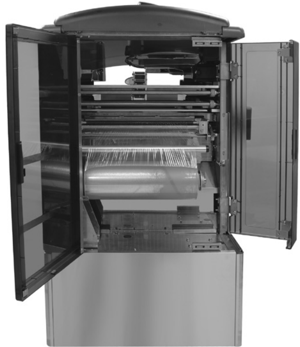
Single roll of film loads in back
