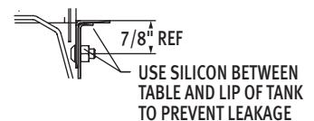
Sectional View Showing Table Connections
