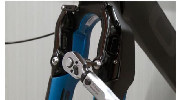
14. Fix brake arm with 6 Nm torque.
