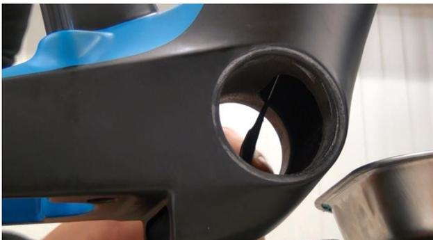
7. Use hook tool to pull help cable out of down tube like shown.
