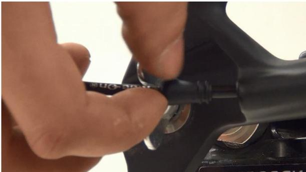
11. When shift cable is installed successfully to frame, put rubber plug on hose and push into cable exit hole (dust & water protection).
