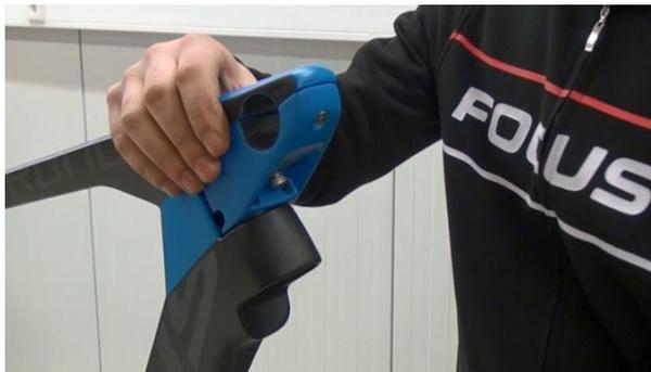
8. Insert stem into head tube's gap. Take care the tooth of aluminum ring catches pocket on rear end of stem.
