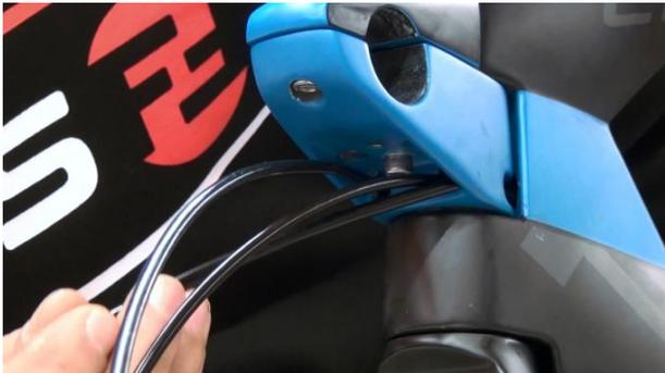
6. Push brake hose through LEFT hand side channel of stem body (in driving direction). It's helpful to twist stem to right hand side when moving brake hose through channel inside frame.
