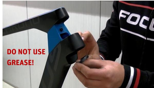
3. Insert lower bearing. DO NOT USE GREASE!
