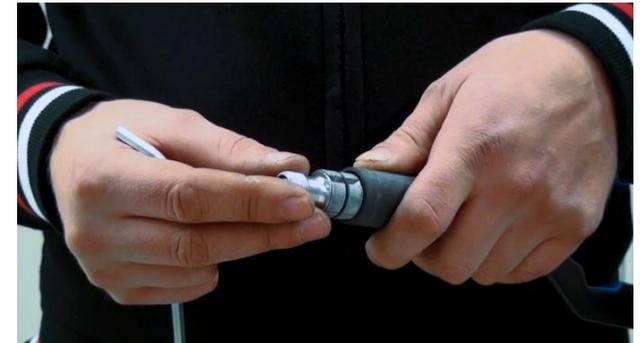
1. Push compressor (together with black cap) into fork steerer. Cap helps to position the compressor at the perfect place.
