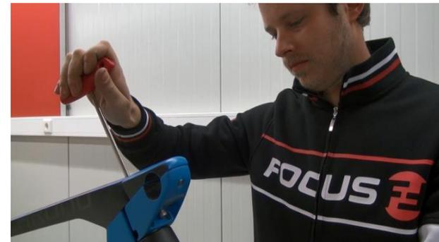
10. Tighten compressor cap (6mm Allen Key) from above with 6 Nm torque.
