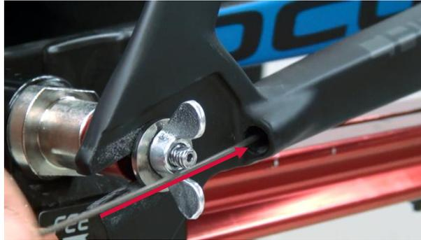
6. Push help cable into chainstay Rear Derailleur cable exit nipple ahead and pull out like shown in next step.
