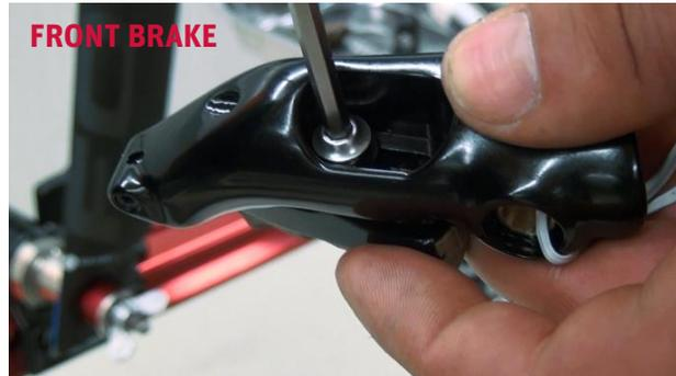
10. FRONT BRAKE: For more convenient installation, detach brake pad.
