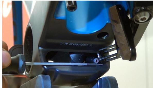
7. Push brake hose through downtube until it reaches the exit behind BB shell. If necessary grab hose with some hook tool.
