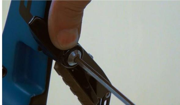
4. Use outer hole position for tension spring (this gives more tension = better performance to rear brake system). Fix with 6 Nm torque.
