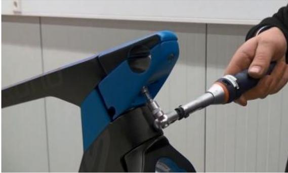
11. When aligned tighten stem with 15 Nm torque.
