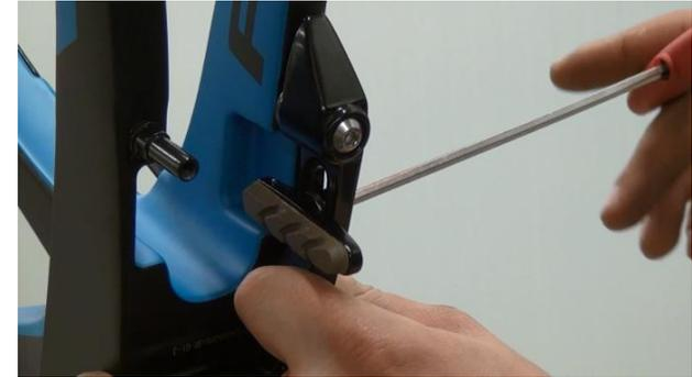
5. Re-install brake pad and tighten with 5 Nm torque.
