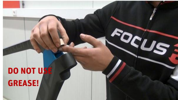
6. Insert IGUS bush bearing. DO NOT USE GREASE!
