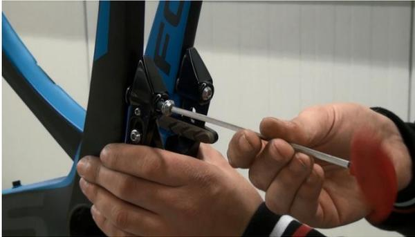
9. Attach left hand brake arm. De-install brake pad first, so hole for tension spring can be found more easily. Use outer hole position for tension spring. Then fix brake arm with 6 Nm.
