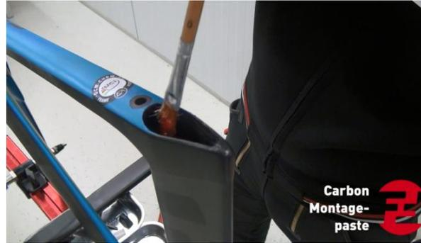
2. Apply friction paste to inner wall of seat tube. Don't use too much paste as this would decrease friction!
