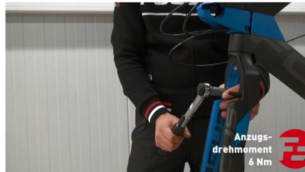
1. Mount all cantilever sockets to frame/ fork with 6 Nm torque.
