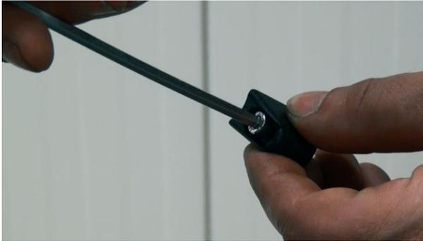
1. Prepare Seat Post Clamp Cone by pre-installation of screw. Clamp cone can be very loose.
