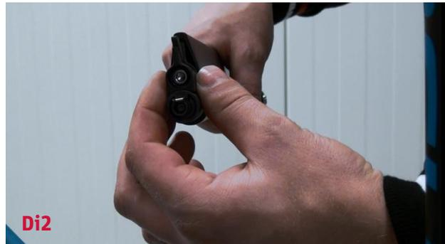
Optional: Put Di2 battery and fixation device (d1) into seat post together in one step. Align battery according to your demands (depth).
