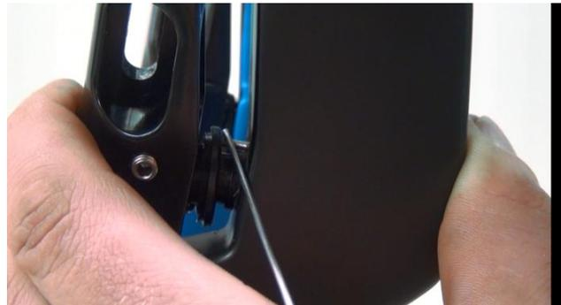
13. Use some hook tool for tension spring attachment/positioning.
