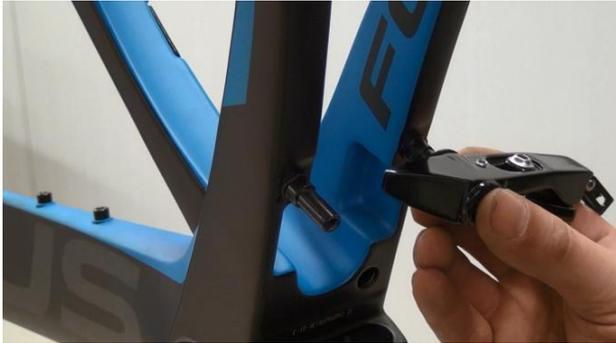
3. Place brake arm on cantilever socket.
