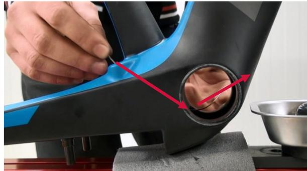
1. Push help cable (shift cable you won't use later) nipple ahead through hole on Chainstay and pull out from inside BB shell.
