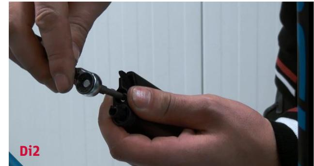
Tighten Di2-fixation with Allen Key.
