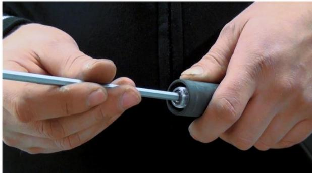
2. Twist off black cap and tighten compressor with 8 Nm torque. Take care compressor is centered in the steerer. Upper end must be flush with steerer end.
