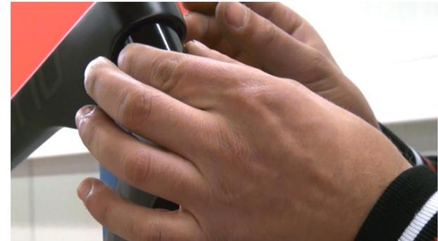
7. Put black aluminum ring (toothed) and compressor cap together and insert into upper part of head tube. Tooth of aluminum ring must point towards frame (to back) and face down.
