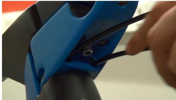
12. Front Derailleur Cable is moved and guided through left hand side channel of stem. Push cable hose through downtube until BB shell.
