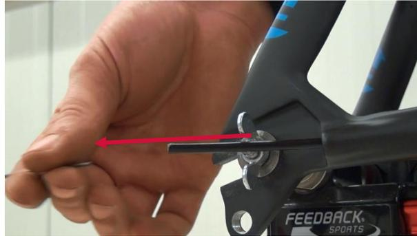
10. Push at front and pull at rear end to move cable housing through the frame.
