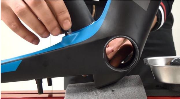
5. Mount Counter Nut to end of Cable Tunnel to fix this.
