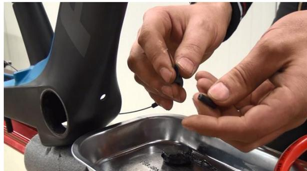
3. Thread Open End Cap onto help cable and plunge it into „trumpet“. Push hard to ensure tight fit and Cap is in right position.
