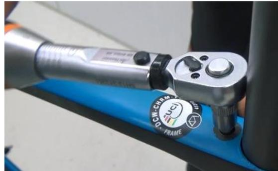
5. Tighten Clamp Cone with 3 Nm torque.
