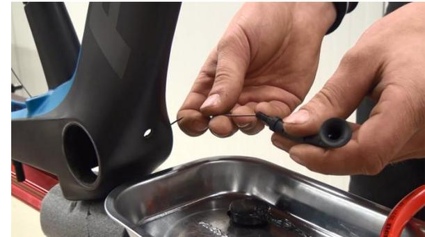
2. Unscrew cap and thread Cable Tunnel onto help cable.
