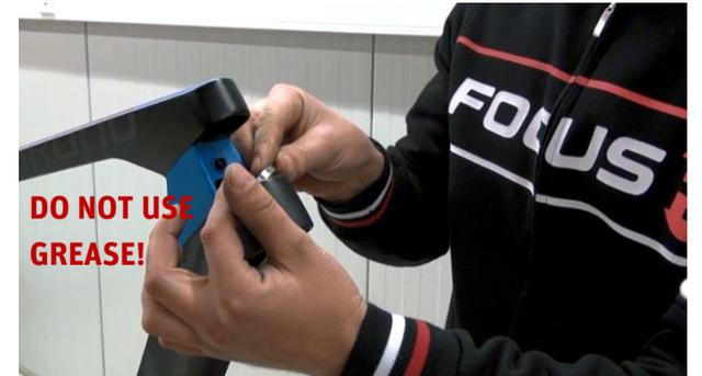
4. Insert upper bearing. DO NOT USE GREASE!
