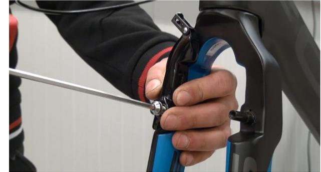
11. Use inner or outer hole position for brake arm tension spring (this is up to you and what feel you want to create for front brake). Fix brake arm with 6 Nm.
