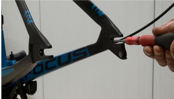
1. Adjust stud screws on both sides according to tire thickness and wheel alignment.
