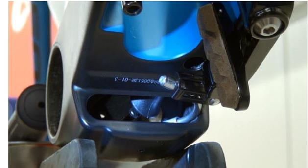
8. Attach Pipe to brake hose. It helps to squeeze pipe body a bit so it cannot detach from hose later. When fixed, push hose a bit back into frame and connect pipe's end to brake arm hanger.
