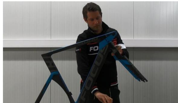
9. Push fork through sterer, bearings and stem from below in one step.
