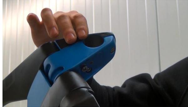
12. Check steer angle limitation on both sides by twisting stem to left and right. Angle must be +/- 45°.
