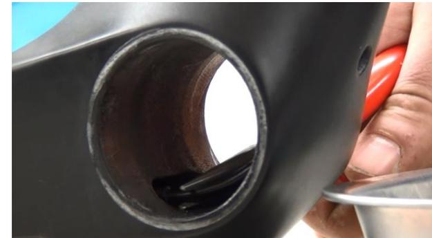
13. Plug end of Front Derailleur Cable Hose tightly into Cable Tunnel (Open End Cap has been pre installed before!). It helps to use some needle-nose pliers for connecting those two parts with each others.
