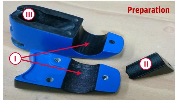
Apply Friction Paste to contact surfaces to handle bar clamp (I), clamp cone (II) and fork steerer contact area (III). Please do not use too much paste as this would decrease the friction. Surfaces should have a „wet look“ without noticeable color off he paste.
