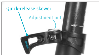
For 1. Quick-release skewer open
