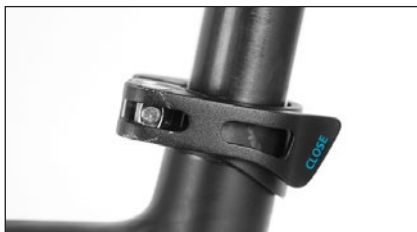
For 3. Quick-release skewer closed
