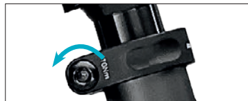
For 1. Loosen seat clamp(s)
