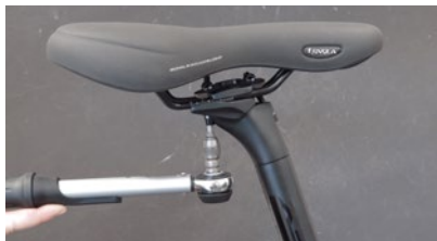
For 1. Loosen screws
