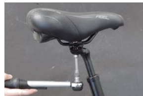
For 1. Loosen the clamping screw
