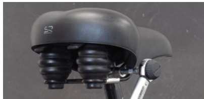
For 1. Loosen clamping nut
