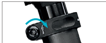
For 3. Tighten seat clamp(s)
