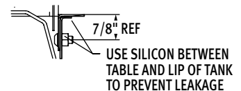
Sectional View Showing Table Connections
