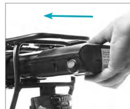
*Reinstalling the battery*
