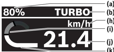
**(a)** State of charge of eBike battery (can be configured)
