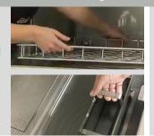
**REINSTALL CLEANED** STRAINER SCREEN(s). scrap basket and rack into the machine and close the door.
