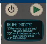
Open the door. Pour deliming chemical into the tank per supplier instructions for a 21 gallon tank (PW10) or for a 34 gallon tank (PW20). Close the
