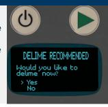
"DELIME INITIATED" will appear on the display. Press 🛍 to enter the delime mode. The machine will drain and refill with fresh water. This will take some time to complete.
