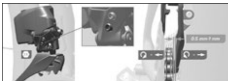
Fig. 97 Setting the upper stop ©Sram
