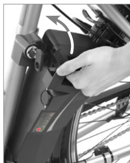
Reinstalling the battery
