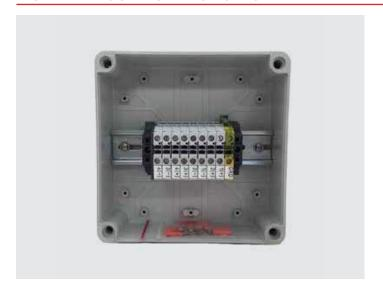
The Solar RU-2-LP Box enables installers to transition and/or combine one to four DC strings to a single conduit, reducing costs by enabling installers to switch to standard building wire and simplifying connections in the enclosure. The low profile enclosure is designed to be mounted beneath the array using the optional box bracket accessory or adjacent to the array using racking system accessories.
