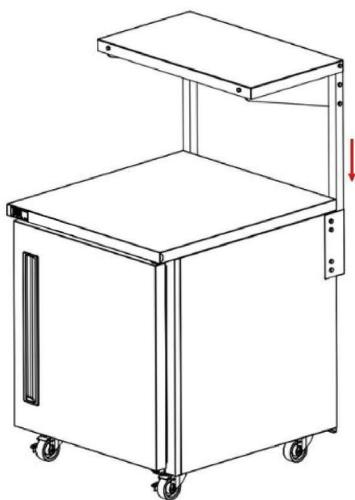
8. APPLY FORCE TO SUPP BRACKETS FORWARD TO ENSURE TUBE IS FLUSH WITH CABINET. TIGHTEN BOLTS WHILE APPLYING FORCE. (BOTH SIDES)
