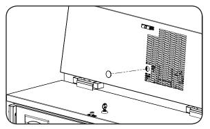
The temperature control is located behind the silver plug on the front side of the system area (dial thermometer side). To adjust, remove the plug turn the adjustment screw with a pair of pliers a small amount at a time; turning clockwise lowers the temperature. An "OFF" position is fully counterclockwise and interrupts power to the compressor and condenser fan only, not the entire refrigerator.
