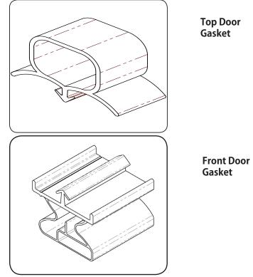
NOTE: System gasket attached with screw.
