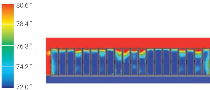
The CFD model shows significant recirculation of exhaust air over the tops of the racks. The color red indicates temperatures exceed ASHRAE TC9.9 recommended temperature of 80.6 Deg F.
