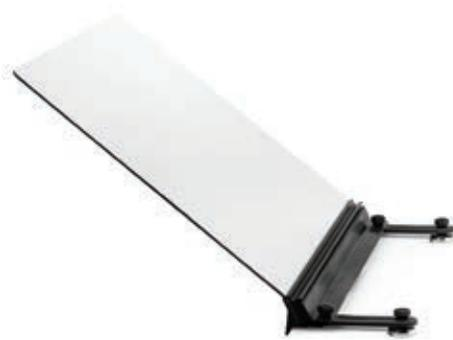
Typically installed on the top front edge of an IT rack in a cold aisle. The Rack Top Baffles extend from the front edge of the rack into the aisle, reducing the open area of the aisle and slightly pressurizing the cold aisle relative to surrounding areas. In addition, the Rack Top Baffles significantly reduce the recirculation of hot exhaust air from the rack equipment across the top of the rack and back into the front intake of the rack. These angled baffles cover 66% of the top of the aisle.
