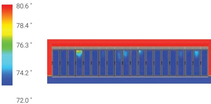
With Proline Express Containment the rack inlet temperatures become very consistent top to bottom, and are all below the ASHRAE TC9.9 recommended temperature of 80.6 Deg F. The maximum reduction in rack inlet temperatures was 10.3 Deg F and the average reduction in rack inlet temperatures was 3.7 Deg F. It is important to note the racks now have uniform inlet temperatures. This enables further optimization of cooling tile airflows and cooling unit operational set point temperatures.
