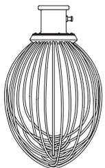
The **D Wire Whip** is designed for maximum blending of air into light products. Uses include: whipping cream, beating egg whites, mixing very light icings, meringues and all similar applications. The D Wire Whip is most commonly used in third and fourth speed.
