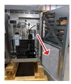
The air filter in all the prep tables is located in the interior of the louver door and does not require any tools for removal (see image to the left).
