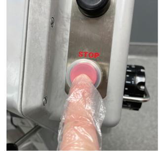
**3. PRESS RED STOP BUTTON.** A built-in brake will quickly stop the attachment shaft when power has been turned off.
