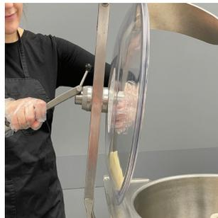
**8. ATTACH BAFFLE HANDLE.** Hold baffle handle with lock knob upright and large knob of baffle handle at bottom, and slide round pin over the mixing baffle shaft and into groove.
