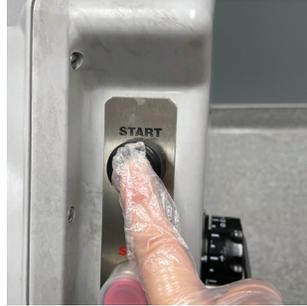
**2. PRESS START SWITCH & RELEASE.** Machine will run until stop button is pressed or, until selected time has expired.
