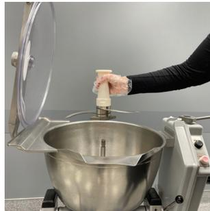
**5. INSERT ATTACHMENT.** Slide attachment onto center shaft. Rotate until it drops down over square part of center shaft. Be sure attachment drops completely into place.
