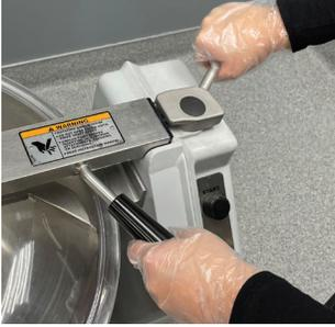
**1. UNLATCH & OPEN COVER.** Wait until shaft has stopped turning.
