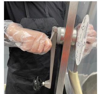
**9. LOCK BAFFLE.** Rotate lock knob downward until it stops.
