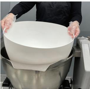
**1. INSERT STRAINER BASKET.** Do not use with mixing baffle.
