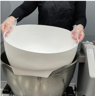
**4. WHEN REQUIRED INSERT STRAINER BASKET.** Place strainer basket into bowl. DO NOT use with mixing baffle.
