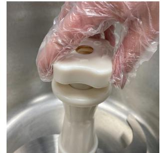
**6. LOCK ATTACHMENT.** Use the twist lock knob furnished. Place knob over shaft and twist until tight.
