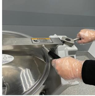
**2. UNLATCH COVER.** Holding cover handle in left hand, pull the cover latch toward you.
