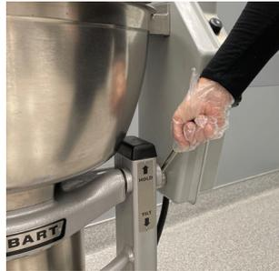
**5. UNLOCK BOWL.** Lower bowl tilt lever to the “Tilt” position.
