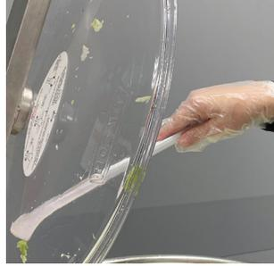
**2. SCRAPE COVER & MIXING BAFFLE.** Cover scraper will remove most product, use a rubber scraper to remove the rest.
