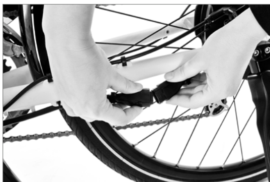
Disconnecting the cable
