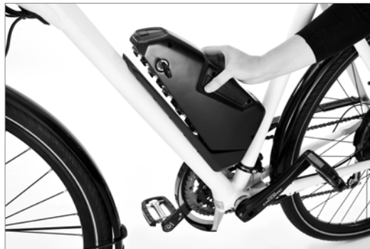
Installing the battery
