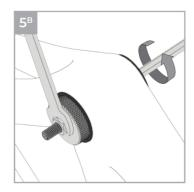
To easily apply more force <u>if</u> <u>the bearing is seized</u>, use a 17mm open spanner on the extractor cup and a long 8mm allen key from the inside on the driver bolt.
