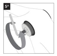
Place a 5mm Allen key on the driver bolt and turn it counterclockwise while holding the cup to extract the bearing from the bottom bracket.
