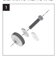
Assemble the tool by placing the correct extractor plate matching your bearing on the driver bolt, followed by the extractor cup.
