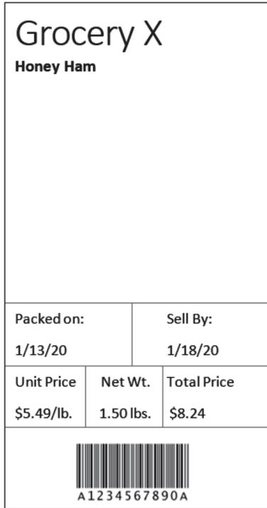
**Die cut labels** are a fixed length and cannot be dynamically sized. The label length is pre-determined by the maximum amount of PLU information to be printed on the label. This results in unnecessary blank label space for those items that require less information printed. (See example).
