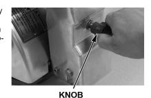
Tilt the Product Tray to the right. The Product Tray can be cleaned in this open position, or it can be removed by grasping with both hands and lifting straight up.
