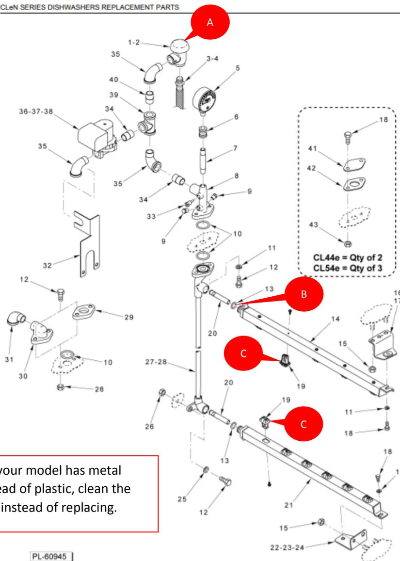
**C - Note:** If your model has metal nozzles instead of plastic, clean the nozzles well instead of replacing.
