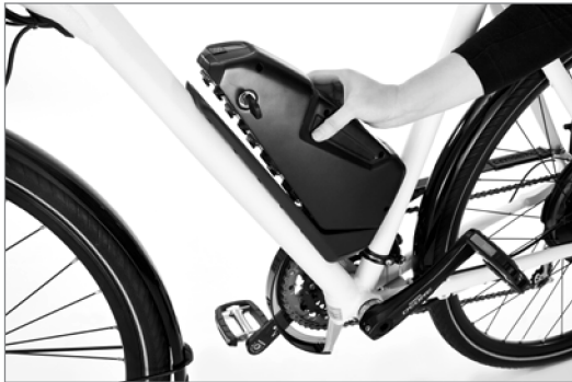
Installing the battery
