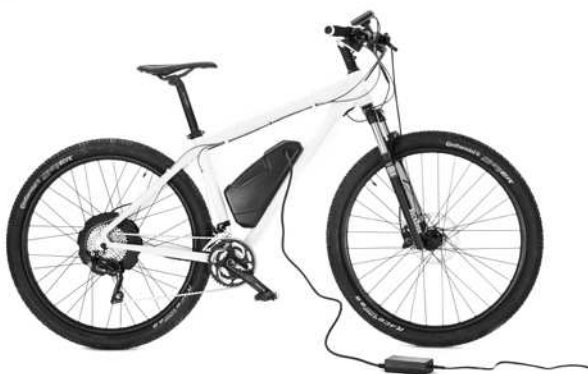
Charging the battery
