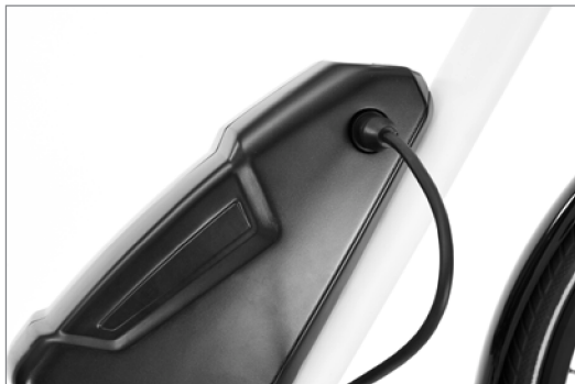
Charging the battery
