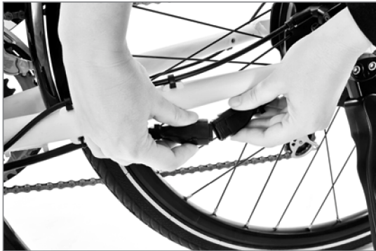
Disconnecting the cable
