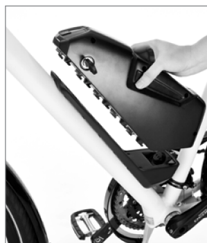
Installing the battery
