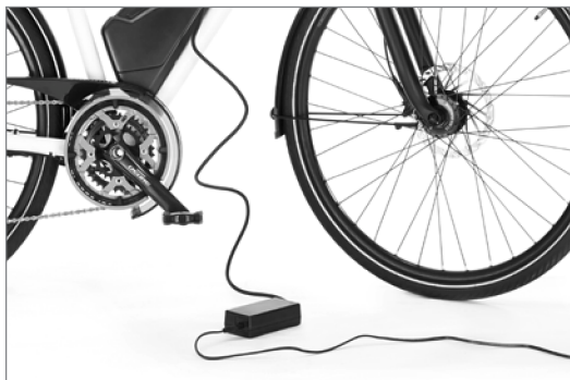
Charging the battery
