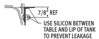
Sectional View Showing Table Connections
