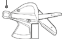
Obr. 61 Zmena napnutia lanka ©Shimano
