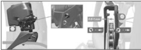
Fig. 96 Setting the upper stop ©Sram
