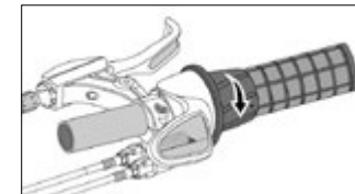
Fig. 102 Shifting to a higher gear ©Shimano
